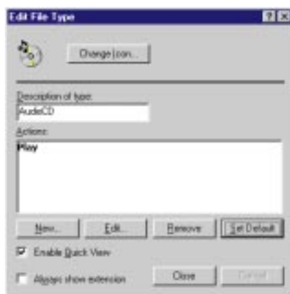
Fig 3 (top) Enabling Autoplay of both CD-ROMs and audio CDs. Fig 4 (above) Audio CDs need this default action, too
